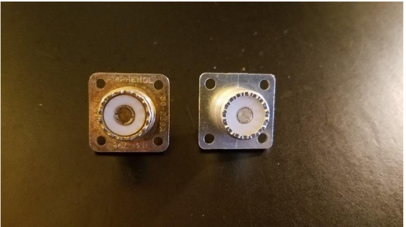
Figure 5. SO-239s. The one on the left is an old Amphenol that is clearly marked. The marks include the manufacturer, the type and the part number – there is zero mystery about what this is. The one on the right is a “mystery” connector. The old Amphenol fits tightly with a PL-259 and is perfectly serviceable. The nice shiny brand new one on the right is junk – a PL-259 slips into it so easily the connection is intermittent.
