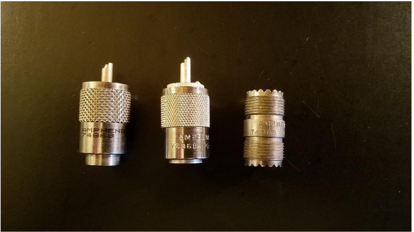
Figure 2. Examples of Amphenol PL-259 connectors. The left one is marked in ink, the centre and right one have their markings stamped into the body. All carry both the name of the manufacturer and a part number. The inked PL-259 is an authentic Amphenol.
